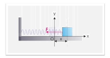
The mass is 300 grams (0.3 kg). The spring has a stiffness given by the constant K = 200 Newtons/meter. The mass is initially displaced 15 cm (0.15 m) from equilibrium. It is held at rest and then RELEASED. The mass therefore starts traveling in—toward the equilibrium position. The equilibrium position is designated x = 0 m.
